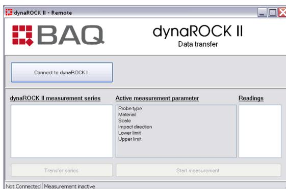
After the connection has been established, the names of the series of measurements saved in the dynaROCK II will be read and displayed in the list 'dynaROCK II measurement series'. The active measurement parameter will also be read and displayed.
