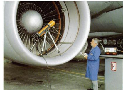
Structural integrity testing in the aerospace segment, where special materials, honeycomb sections and composites demand exceptional tube performance.
