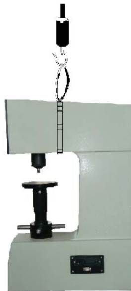
Figure 3-2 Lift the testing machine
