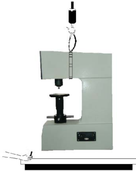
Figure 3-3 install the leveling screw
