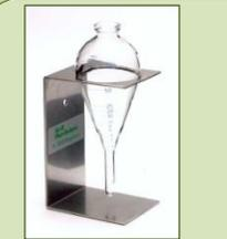
For control concentration of test suspension (especially new preparation) .Sedimentation glass with fine scaling.
