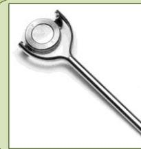
The technical device defines direction of magnetic field and shows incorporated artificial errors.
