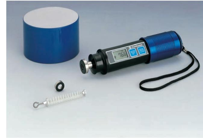
The rebound hardness tester DynaPOCKET contains a display and an evaluation unit, integrated into one instrument, ensuring compact design without any cables and characterized by its small size and light weight.
