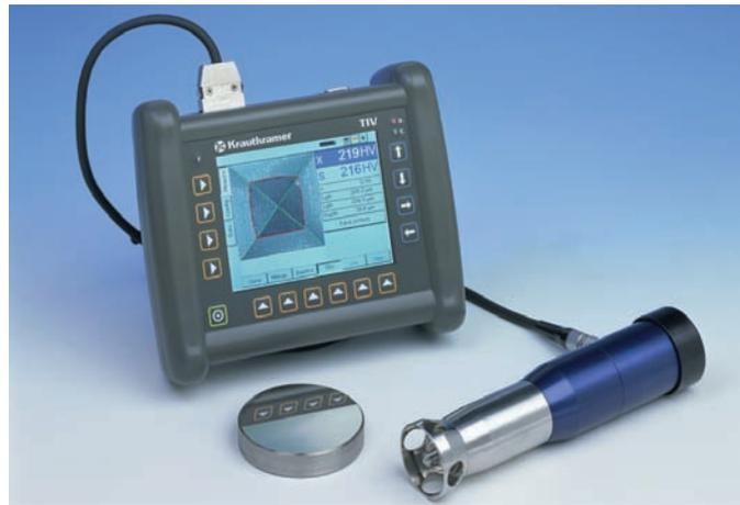
The TIV (Through Indenter Viewing), which is based on hardness testing according to Vickers, can “see through” the indenter – the Vickers diamond – by means of special optics and a CCD camera.
