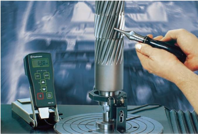
The MIC 10 enables quick and convenient on-site hardness testing according to the UCI method (Ultrasonic Contact Impedance) with a Vickers diamond as indenter.
