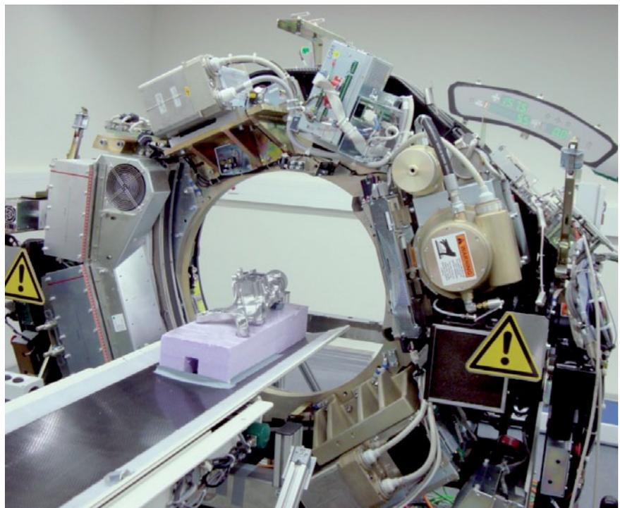
**Figure 2.** Laboratory-scale high-speed CT scanning a die casting
