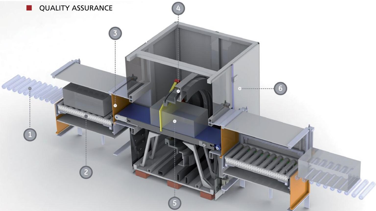
**Figure 14:** High-speed CT system in in-line arrangement: (1) roller table, (2) roller table with lifting system for level adjustment, (3) slide gates (radiation protection), (4) scanning unit (gantry), (5) specimen, (6) radiation-proof cabin
