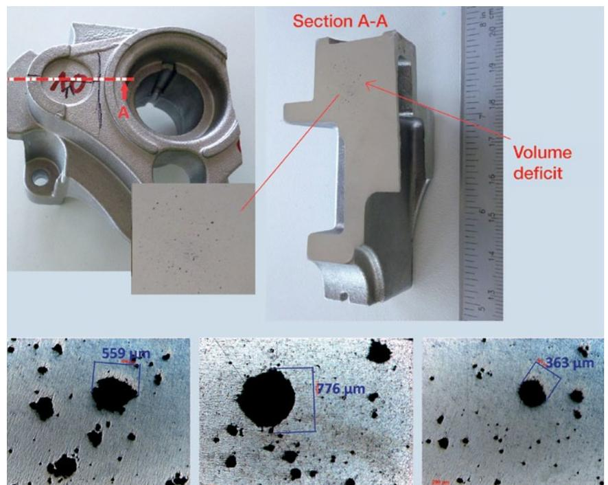
**Figure 10:** Metallographic examination of part No. 10, the part with the lowest porosity in Figure 7b
