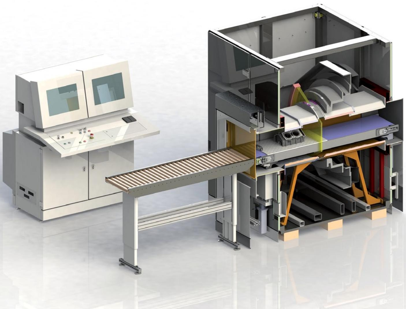
**Figure 13:** High-speed CT system in at-line arrangement
