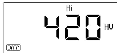
The setting is made in the same hardness scale as selected in **MEASUREMENT** level:
