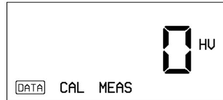
The calibration is retained when the instrument is turned off.
