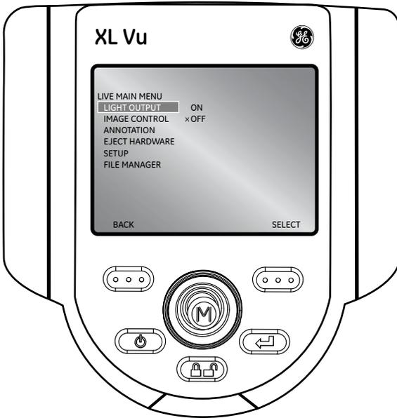
**Note:** Turning on FREEZE FRAME is a convenient way to turn off the light output and is ideal for changing optical tips. For Battery models this also conserves battery charge.
